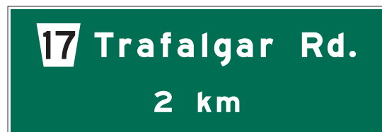
(a) G103 – Freeway Pre-Advance Sign
