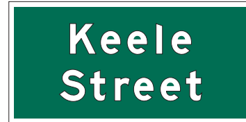
Figure 5.28: G220 – Roadway Identification (Grade Separation) Sign
