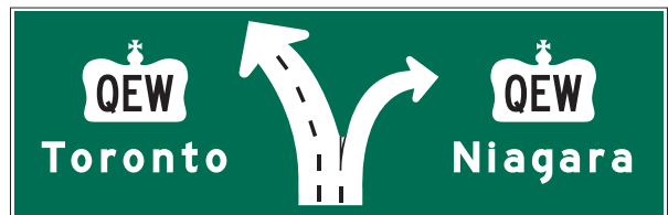
Figure 5.12: G102 – Freeway Diagrammatic Pre-Advance/ Advance Sign
