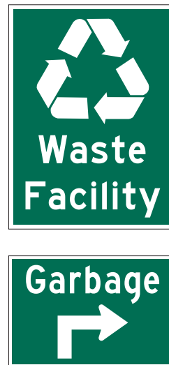
Figure 13.11: Waste Management Facility Sign and Optional Tab
