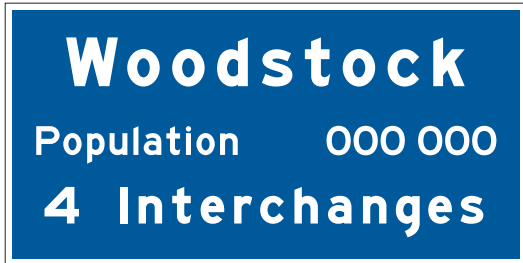
Figure 5.20: G312 – Multiple Interchange Boundary Sign (1-9 Interchanges) (Basic)
