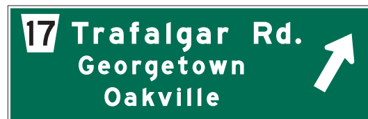
Figure 5.2: G101 – Freeway Turn-Off Sign (Ground-Mounted)
