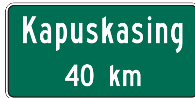
Figure 8.25: G303 – Auxiliary Assurance Sign
