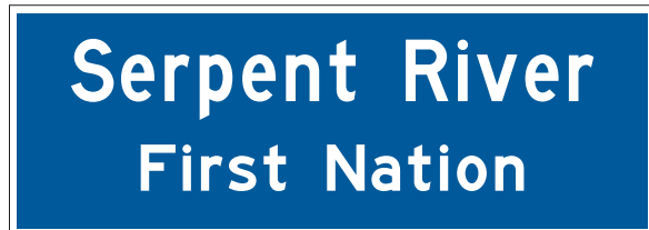
Figure 5.19: G320 – Boundary Sign – First Nations (Basic)
