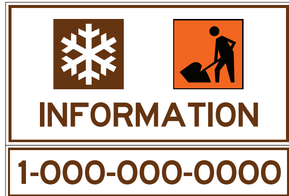
Figure 13.14: G700 – Highway Conditions and Construction Information Sign
