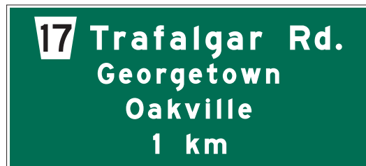
Figure 5.4: G100 – Freeway Advance Sign (Ground-Mounted)
