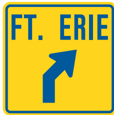
(e) M201 – Combined DESTINATION and Direction Marker (used with QEW marker only)
