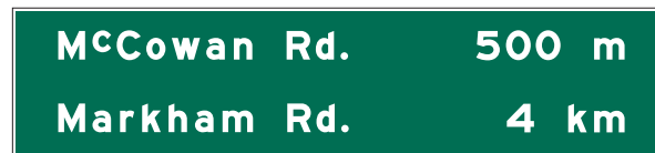
Figure 5.13: G112 – Freeway Interchange Sequence Sign
