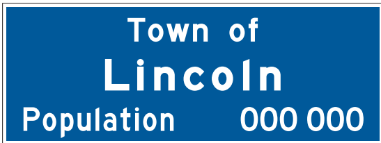
Figure 5.17: G314 – Boundary Sign – Single-Tier/Lower-Tier (Basic)
