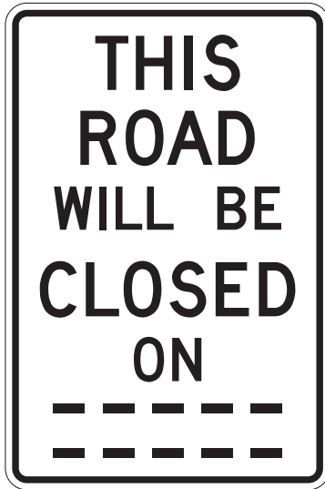
Figure 17.9: G725 – Notice – Road Closed (with Date)
