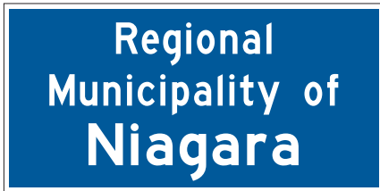
Figure 5.16: G318 – Boundary Sign – Upper Tier - 3 lines (Basic)
