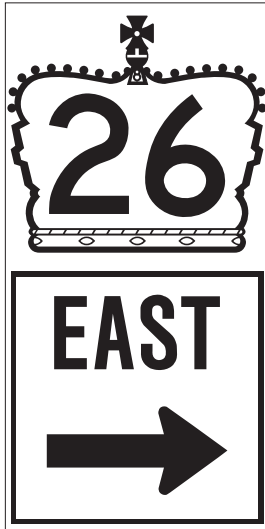
(b) M114 - Combination Marker - Provincial Crown with Cardinal Direction and Arrow
