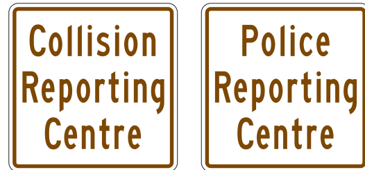
Figure 11.8: M405 – Collision/Police Reporting Centre Marker
