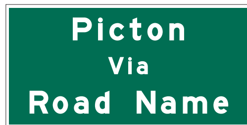
Figure 5.27: G309 – Supplementary Destination Sign
