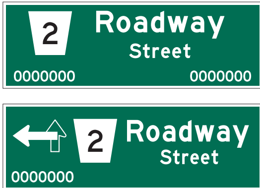
Figure 11.1: Example of Turn-Off Sign with 911 Information
