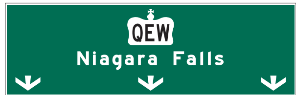
Figure 5.14: G113 – Freeway Pull-Through Sign
