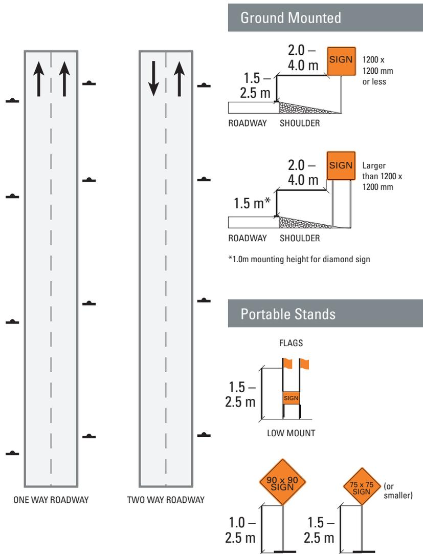
The objective is to place the signs in the driver's cone of vision.
