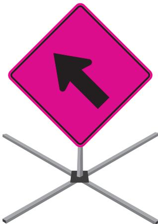
First responders may carry flexible, roll-up signs with the EMERGENCY SCENE AHEAD message or directional arrow that can be set up quickly at an incident site using portable lightweight spring stands or other appropriate temporary mounting.
