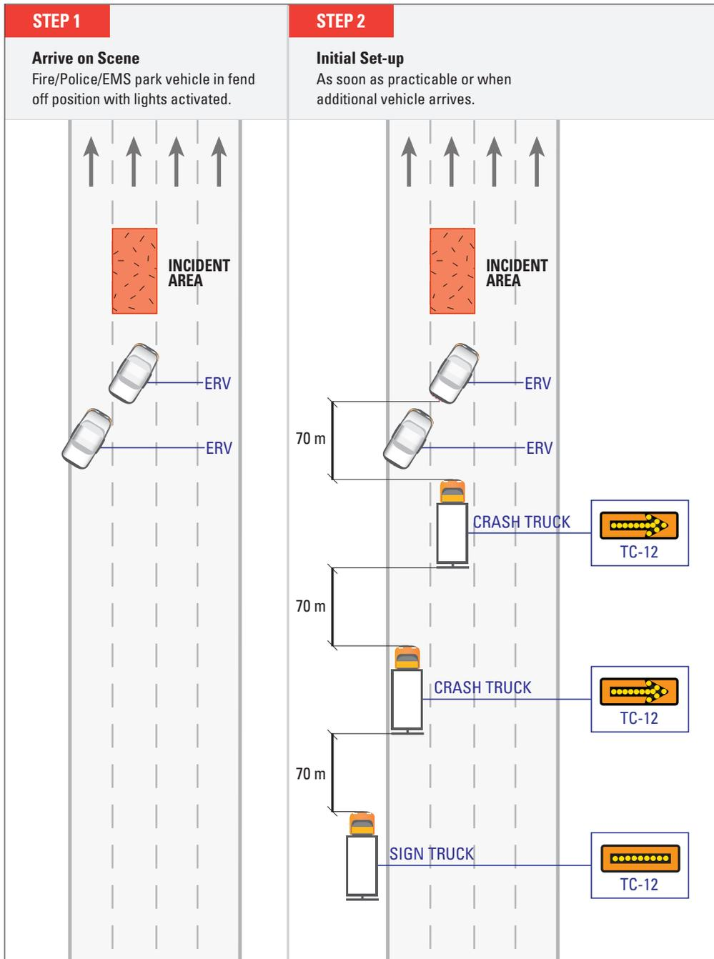
Figure A.8 Typical Setup of Incident in Live Lane (Freeway)
