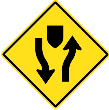
DIVIDED ROAD BEGINS Sign
