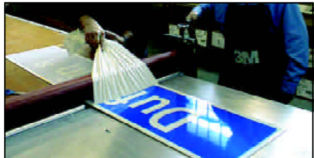
Figure 4.28 – Removal of Transfer Tape
