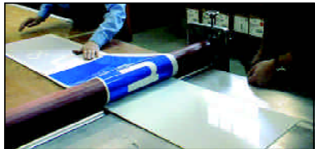
Figure 4.27 – Application of Transfer Tape and Reverse-cut Transparent Sheeting to Reflective White Background Sheeting on Substrate
